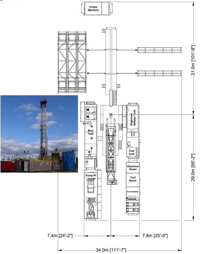
Quantity of pipe tubs in the layout may vary due to customer requirements.
