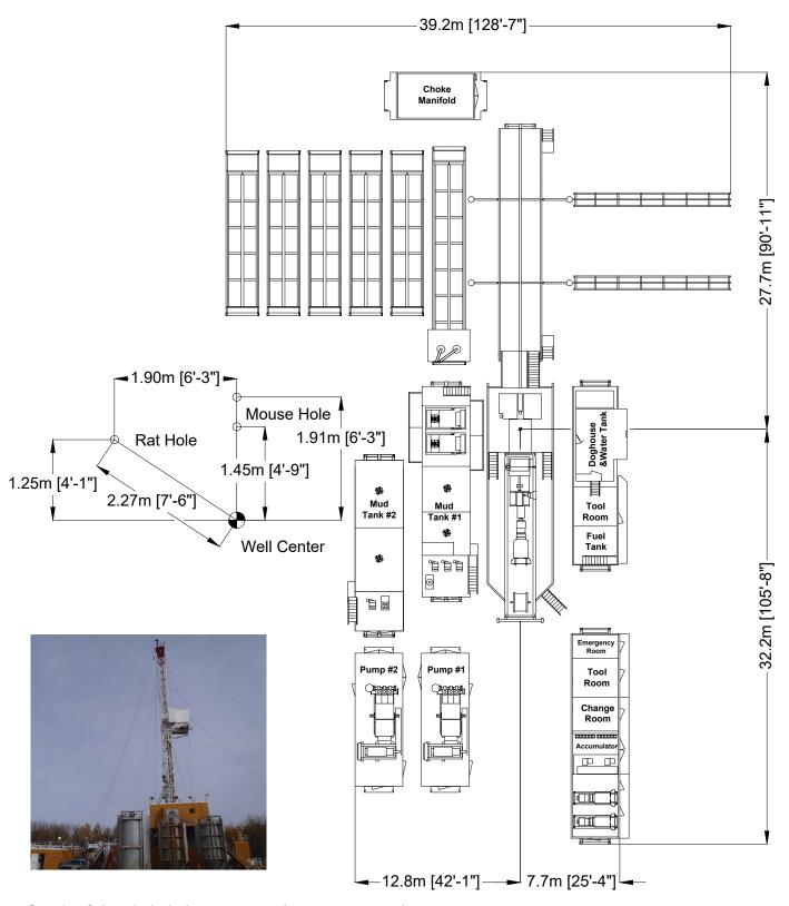
Quantity of pipe tubs in the layout may vary due to customer requirements.
