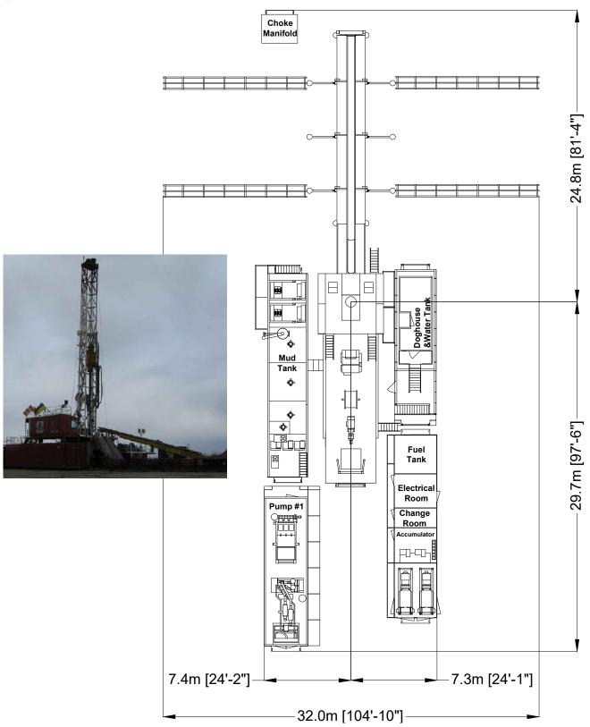
Quantity of pipe tubs in the layout may vary due to customer requirements.
